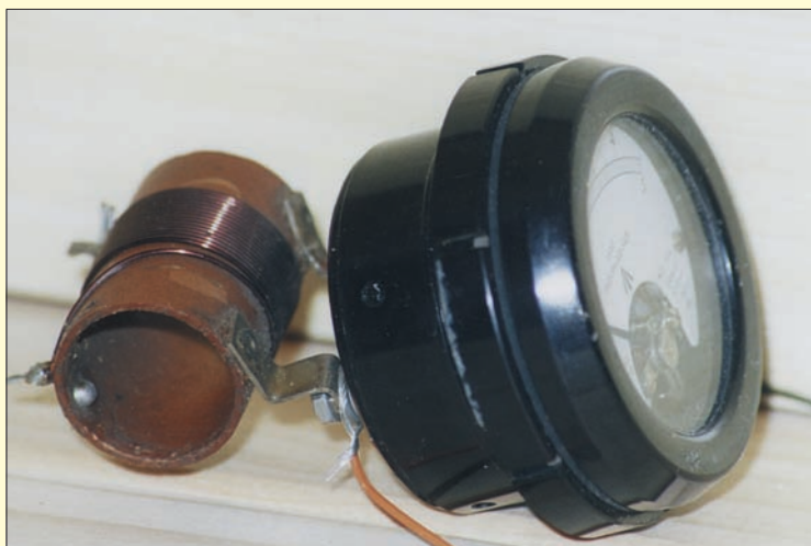
Fig. 2: A meter being prepared for use as a voltmeter. Three high quality wirewound resistors have been chosen to obtain the highest accuracy possible (see text).
