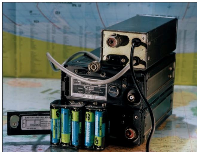
● Fig. 1: The TR-2300 can operate off internal NiCad batteries, a 12V (nominal) external source and dry batteries. If dry batteries are used - a dummy cell has to be employed to reduce the voltage (see text).
